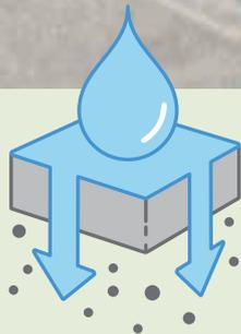
Permeable pavers look similar to traditional pavers but are designed with special spacer bars that create a wider joint.
