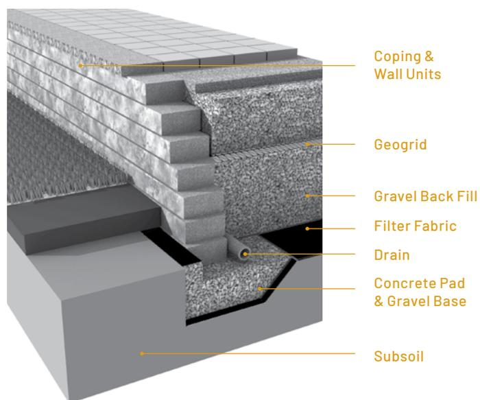
A proper base ensures that your pavers and walls won't shift during freeze/thaw cycles.
